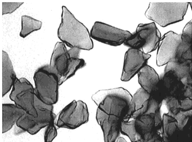
Figure 19. Optical microscopy of functionalized 1000 Å CPG (photograph courtesy of Biosearch Technologies, Inc.).
