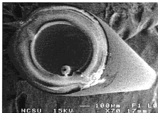
Figure 17. Single Pelican bead in electro-spray nanoprobe needle.
